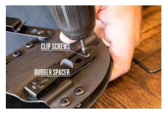
Locate the screws attaching the clips to the holster.
