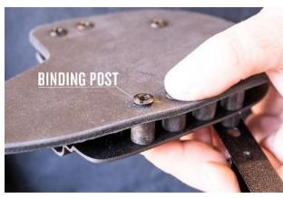
Tighten the screws; locking the clip in place.
